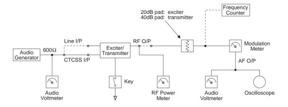
Figure 3.2 T856/857 Test Equipment Set-up
