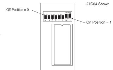
Figure 3.1 Channel DIP Switch Setting
